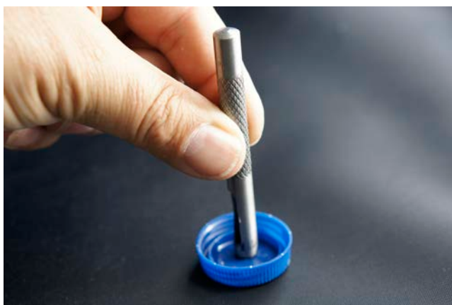
Fig. 51: Example of method for punching holes in bottle caps
